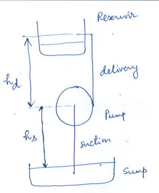
$g(-w) = (p_{+}(\frac{v_{1}}{2}+g_{2}) - (p_{+}\frac{v_{1}}{2}+g_{2}),$  $H_{m} = h_{s} + h_{s}f + h_{d} + h_{d}f + \frac{V_{2}^{2}}{2g}$  $\eta_{\rm h} = \frac{H_{\rm m}}{H_{\rm h}} = \frac{H_{\rm m}}{\frac{U_{\rm h} v_{\rm u_{\rm h}}}{q}}$
