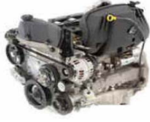
General Motor's inline-5 engine which uses aluminum alloy A356-T6 as its engine block
