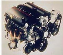
The Chevrolet Corvette LS1 V8 engine which utilizes an aluminum alloy 319-T5 cylinder block
