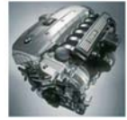
BMW's 6-cylinder R6 powerplant uses a magnesium alloy AMC-SC1-fabricated cylinder block
