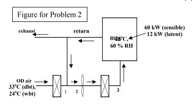
factor of **0.6** is used to cool and dehumidify the outside air only, while Coil 2 handles only sensible load (sensible heat factor = 1.0). If the temperature of air supplied to the conditioned space is **12°C**, find the latent and sensible cooling capacities of Coil 1 and 2. Show the complete process on psychrometric chart. **(6+2 = 8)**
