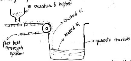
[5th]: To initiate the silicon ingot formation process, we would use the same method as the original czochralski's process of initiating the ingot formation by introducing a pure Si verystal seed. We would dip that seed into that meth and start pulling it up with rotation
