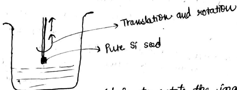
**Step 3:** Perhaps the most difficult step would be to rotate the ingot and pull it up continuously. The translation can be easily done, but the rotation causes a challenge. A proposed mechanism is
