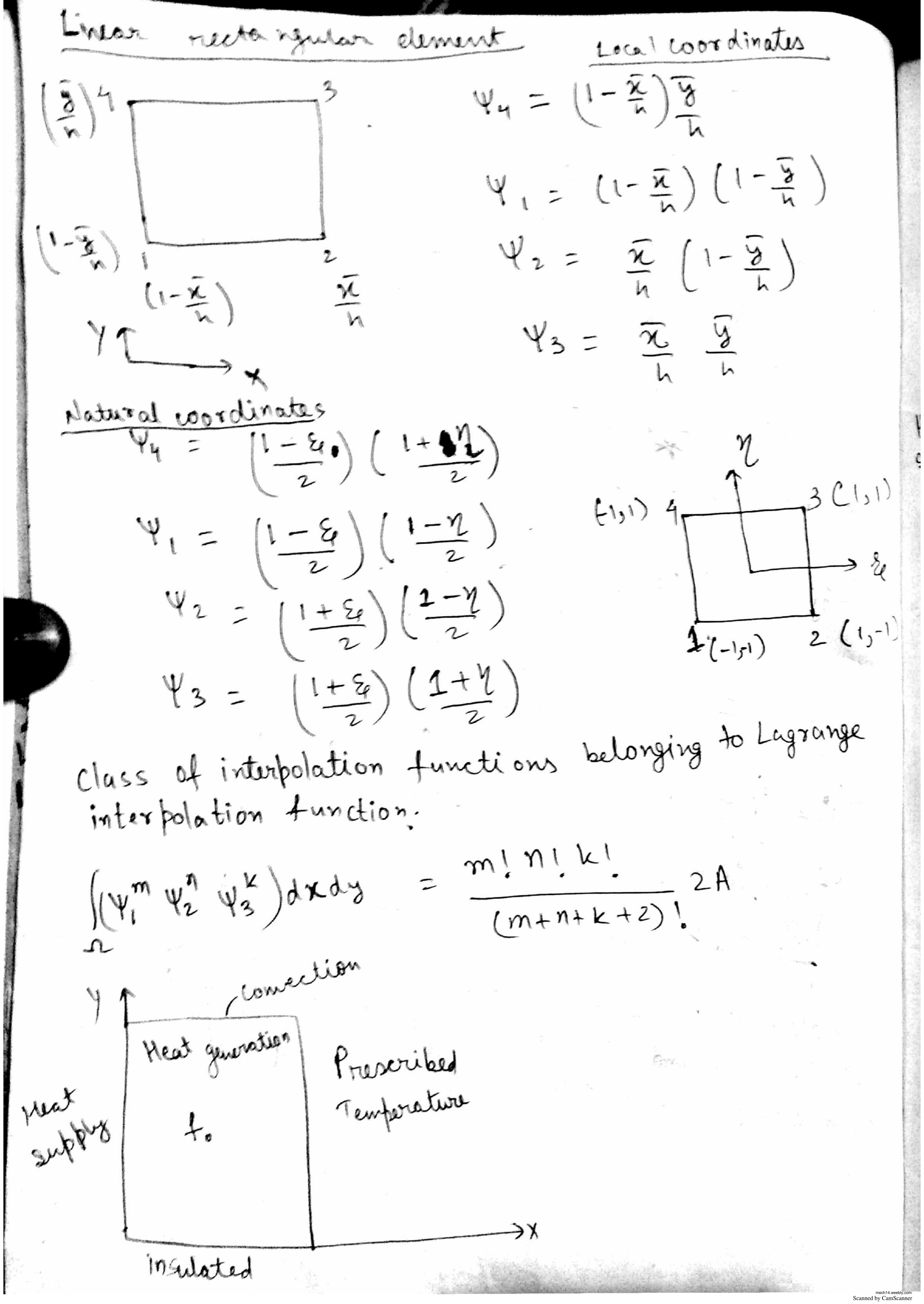
$$-\frac{\partial}{\partial x} \left( k_{x} \frac{\partial T}{\partial x} \right) - \frac{\partial}{\partial y} \left( k_{y} \frac{\partial T}{\partial y} \right) = f(x, y)$$
