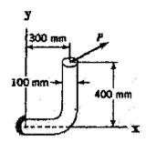
4. The curved beam in the figure below has a 30-mm square cross section and radius of curvature R = 65mm. The beam is made of a steel for which E = 200 GPa and v = 0.29. If P = 6 kN determine the deflection of the free end of the curved beam in the direction of P using energy method and taking into consideration shear, bending and axial load.
