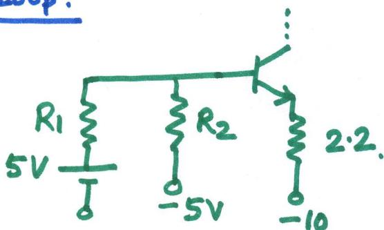
$$V_{TH} = \frac{10R_2}{R_1+R_2} - 5$$
