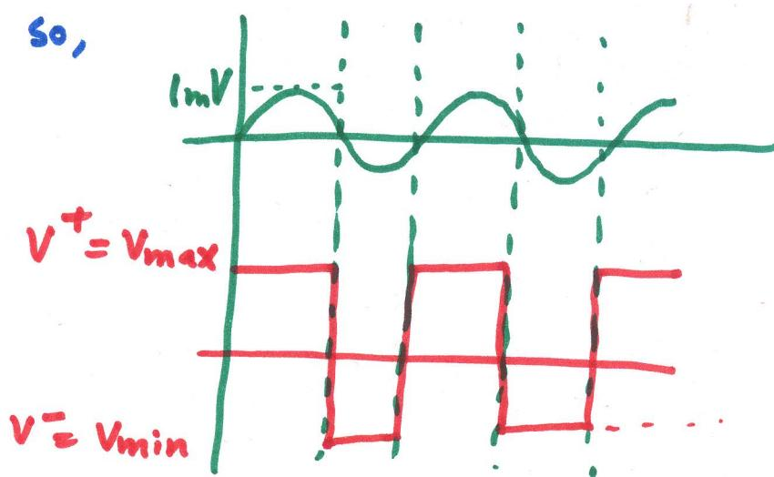
← Applied to the non-inverting terminal (+)
